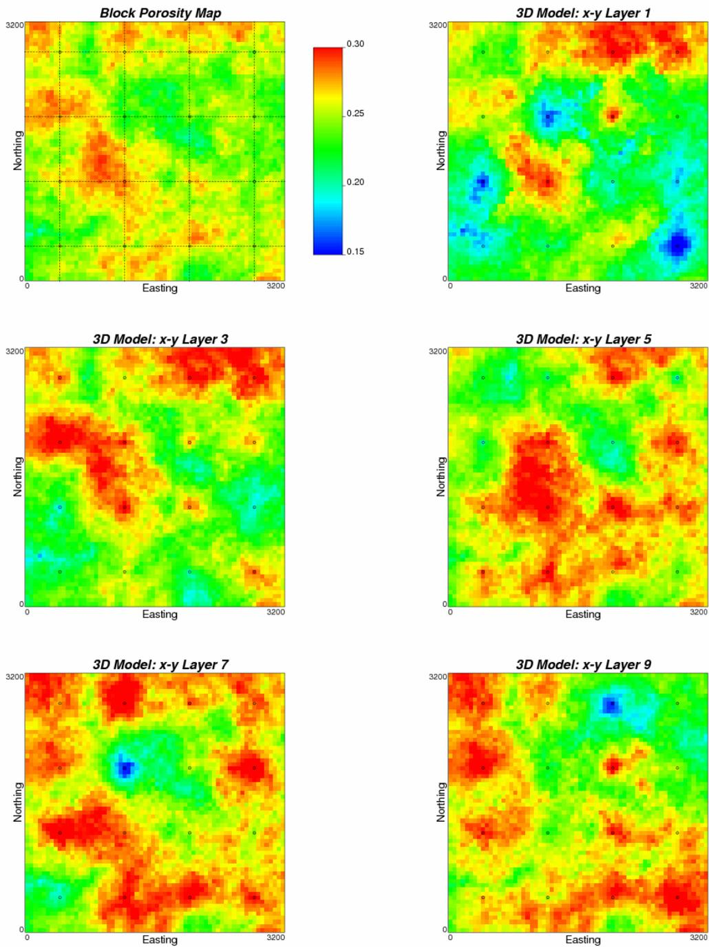
**Figure 9:** The 2-D porosity map and all odd number x-y view slices of the 3-D model from EDDK. The 3-D porosity is at scale of 50x50x1m. The dash lines in the porosity map (the top left) indicate the locations of the x-z and y-z cross sections.
