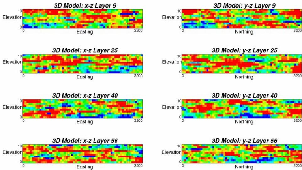
**Figure 12:** The x-z and y-z cross sections of the 3-D porosity model from EDDSS. The 3-D porosity is at scale of 50x50x1m. The dish lines in the x-z and y-z cross sections indicate the wells. The horizontal continuity matches the well data.
