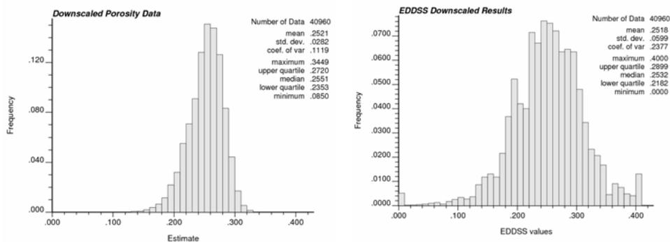
**Figure 14:** The histogram of fine scale porosity estimates from EDDK (left) and EDDSS (right).
