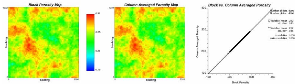
**Figure 13:** The block 2-D porosity map (left), the map of the column averaged porosity from the 3D model (middle), and the cross plot of the two grids.
