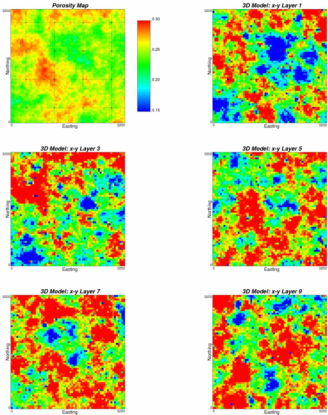
**Figure 11:** The 2-D porosity map and all odd number x-y view slices of the 3-D model from EDDSS. The 3-D porosity is at scale of 50x50x1m. The dash lines in the porosity map (the top left) indicate the locations of the x-z and y-z cross sections.
