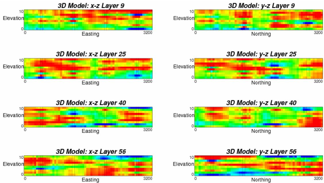
**Figure 10:** The x-z and y-z cross sections of the 3-D porosity model from EDDK. The 3-D porosity is at scale of 50x50x1m. The dish lines in the x-z and y-z cross sections indicate the wells. The horizontal continuity matches the well data.
